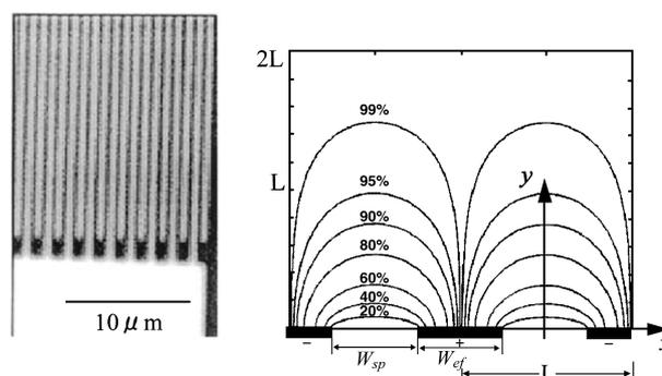
FIG. 4. SEM of IDE and calculated current distribution of IDE. A curve of, e.g.,  $80\%$  means that  $80\%$  of the current flows beneath the curve (15).
