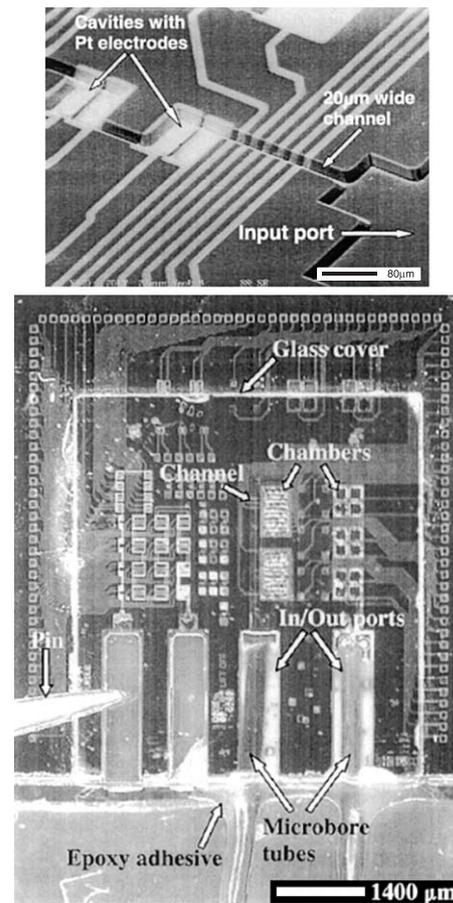
FIG. 7. Scanning electron micrograph of the biochip channels with integrated electrodes and the picture of the completed microfluidic biochip (43).
