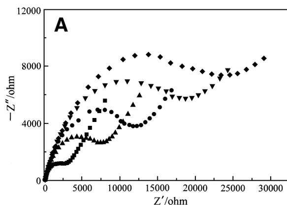
FIG. 3. A layer-by-layer construction of avidin/biotin-labeled-antibody on gold surface and complex plane impedance plots of avidin/biotin-labeled-antibody with increasing numbers of outermost bio-Ab layers from 1 to 5 at  $0.24$  V vs Ag/AgCl in  $10$  mM PBS +  $0.15$  M KCl +  $5$  mM  $[\text{Fe}(\text{CN})_6]^{4-/3-}$  solution. Frequency range is between  $0.1$  and  $100,000$  Hz with a signal amplitude of  $50$  mV (13).
