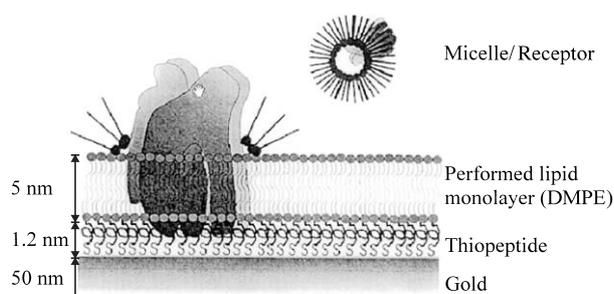
FIG. 1. The incorporation of cytochrome *c* oxidase in a preformed lipid bilayer (7).
