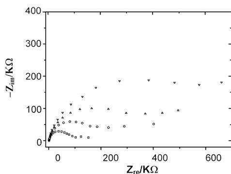
FIG. 2. Complex plane impedance plots for an antibody modified electrode at a potential of  $-1.4$  V vs SCE and AC signal of  $5$  mV, in PBS (squares), without antigen injection; after antigen injection at different concentrations: circles,  $10$  ng/ml; positive triangles,  $50$  ng/ml; inverted triangles,  $100$  ng/ml (11).
