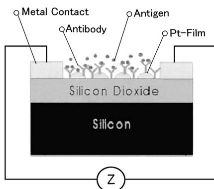
FIG. 5. Cross-sectional diagram of ultrathin platinum film immunobiosensor (16).
