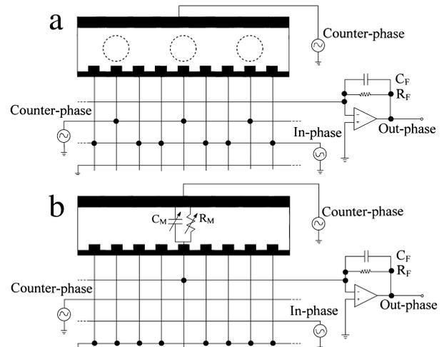
FIG. 8. Circuit connections of the electrodes and the lid: (a) during the actuation, each electrode can be connected, under software control, to an in-phase or a counter-phase stimulus. (b) During the sensing phase, one electrode, with which the measurement is to be performed, is connected to a trans-impedance amplifier and all the other electrodes are connected to the GND; a sinusoidal stimulus is applied to the lid (44).
