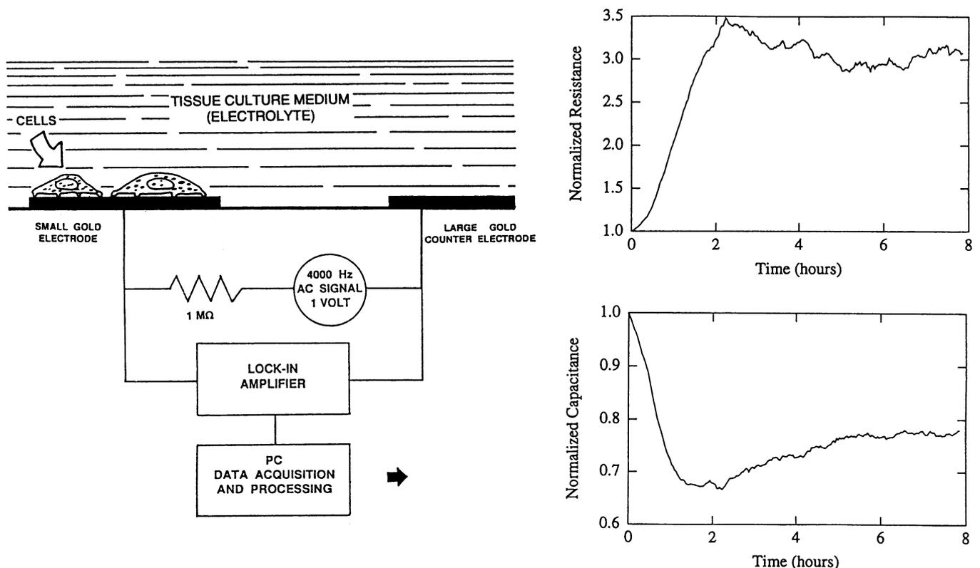
FIG. 3. (Left) Schematic of the basic setup to measure the impedance of primary human fibroblast culture monolayers. (Right) Data concerning the changes in normalized resistance and capacitance accompanying cell attachment to the substratum. These values are calculated by treating the cell-electrode system arbitrarily as a series resistance-capacitance circuit.
